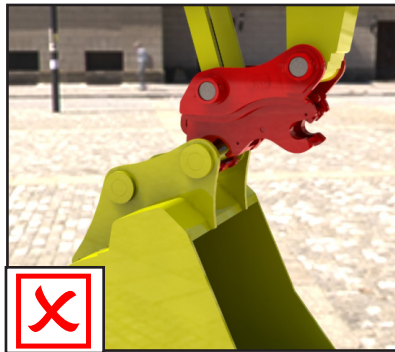
Moving or lifting attachments by front pin only
