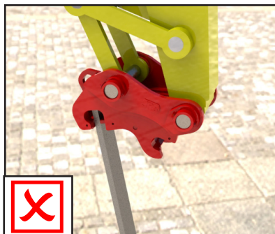
Using coupler to position or hammer objects into the ground
